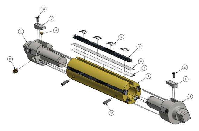
Third Step - Check if Air Bladder(s) are leaking by spraying soapy water on air shaft. Click on hyperlink and view "Air Shaft Troubleshooting & Repair" video on YouTube https://youtu.be/hR4xTYCxAjU
