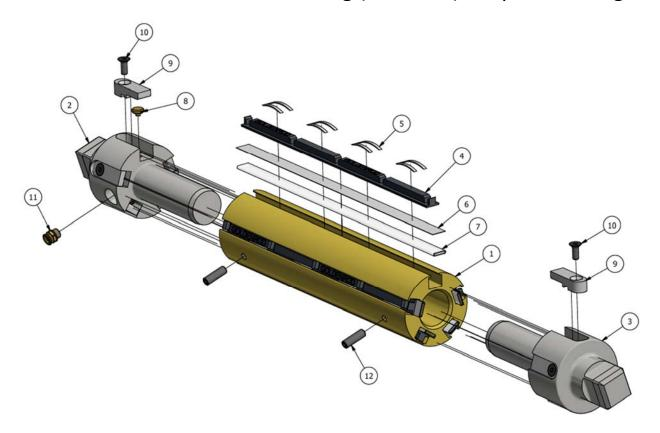
Third Step – Check if Air Bladder(s) are leaking by spraying soapy water on air shaft. Click on hyperling and view "Air Shaft Troubleshooting & Repair" video on YouTube https://youtu.be/hR4xTYCxAjU
